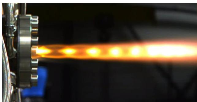
**Exhaust plume during a firing test on PERGOLA**
